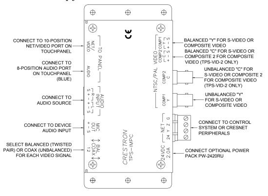
**NOTE:** The included AUDIO cable has a connector with a blue cover to match the blue connector on the TPS-IMPC. As older AUDIO cables may not have the blue cover, be sure to insert the AUDIO cable into the AUDIO port.
